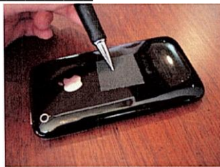
Cell Phone: A Battery Strip (covered with gaffer's tape) has been placed over the battery area of a cell phone
